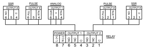
Figure 2.2 Rear Panel Power and Output Connections
